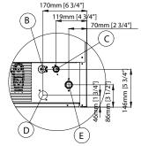
Water outlet connection water condensation 20 mm
