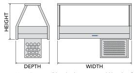
Note: For overall height dimensions, add height of motor cage (450 mm).  $\,$
